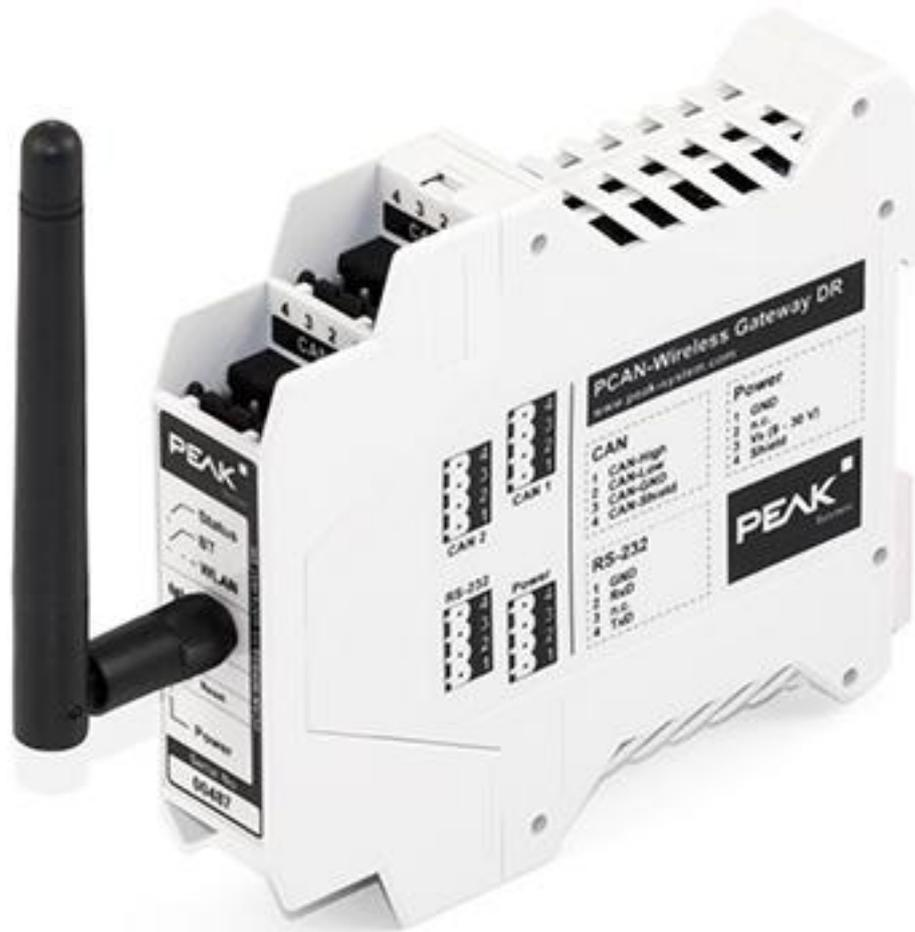
The PCAN-Wireless Gateway DR allows the connection of different CAN busses over IP networks. CAN frames are wrapped in TCP or UDP message packets and then forwarded via the IP net from one device to another. The PCAN-Wireless Gateway DR provides one WLAN connection and two High-speed CAN interfaces. With its DIN rail casing and the support of the extended temperature range, the module is suitable for use in an industrial environment.
