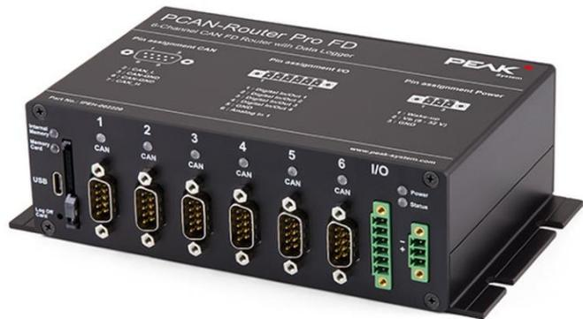
The behavior of the PCAN-Router Pro FD can be programmed freely for specific applications. The firmware is created using the included development package with GNU compiler for C and C++ and is then transferred to the module via CAN. Various programming examples, such as message forwarding or recording, facilitate the implementation of own solutions.
