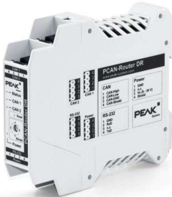
The PCAN-Router DR has two High-speed CAN channels. Their bit rate is adjusted with a rotary switch on the device front. The module forwards the message traffic bi-directionally 1:1 between both connected CAN busses. With its DIN rail casing and the support of the extended temperature range, the module is suitable for use in an industrial environment.
